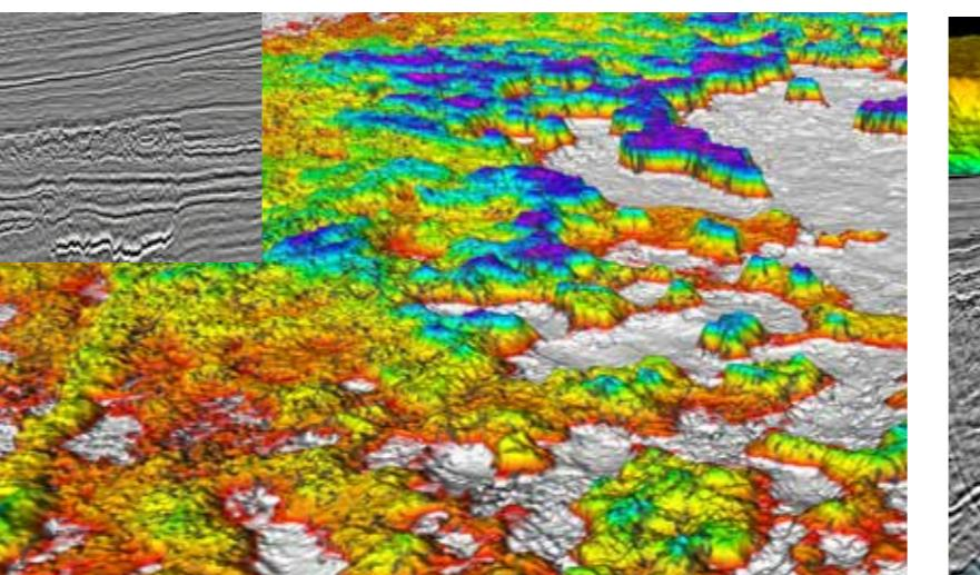
8. New play model for the southern Møre Basin: In the slope down from Tampen we interpret a vast area of Eocene sand injectites. The biggest communicating injectites are  $>50 \text{ km}^2$  and have a soft amplitude anomaly in the top. Interpreted top of injectite facies showing time thickness of facies blended with facies variance. Inset shows intrusive geometry of facies in profile.
