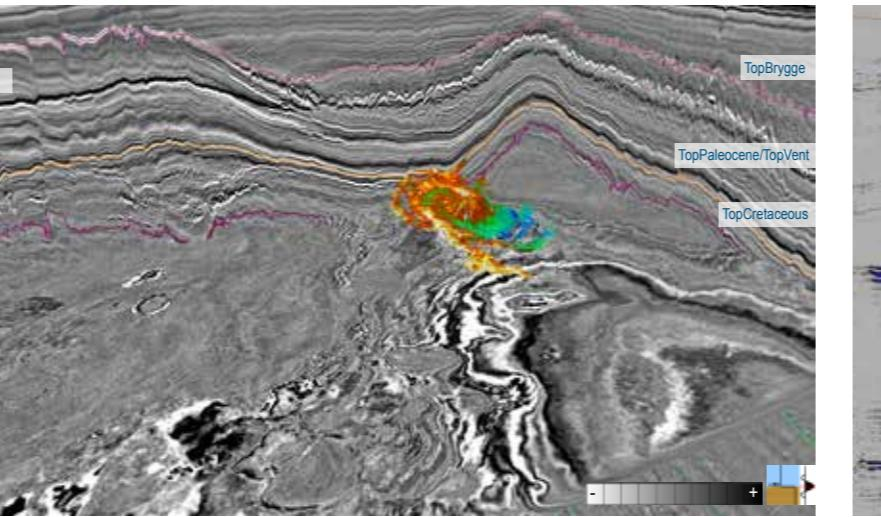
3. One of many anomalies within the Eocene package west of Helland Hansen dome. This  $65 \text{ km}^2$  size lead sits in the syncline between the "Middle dome" and the Modgunn Dome to the left. The amplitude anomaly corresponds to a structural trap created by a hydrothermal vent system from a deeper volcanic sill intrusion.
