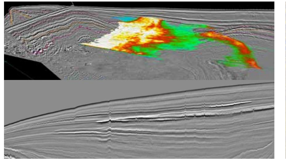
1. New shallow play model: In a vast area ( $>2,500 \text{ km}^2$ ) west of the Helland-Hansen dome we have stacked bright events in the Upper Miocene and lower Plio-Pleistocene package. Phase-inverse amplitude reflections should represent shallow gas below the gas hydrate stability zone. If it is possible to produce from these units, then the volumes of gas present could be huge.
