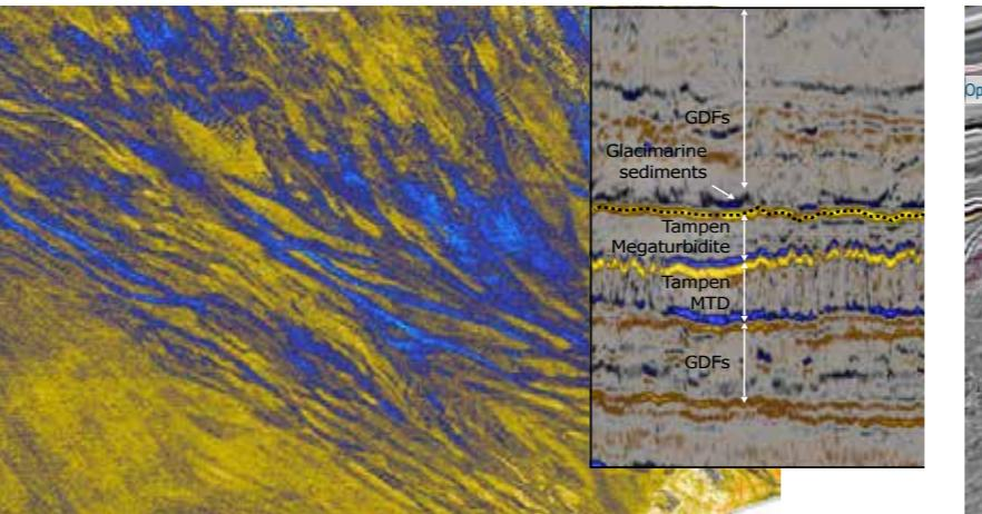
2. New shallow play model: Shallow gas accumulations in glaci-marine sands deposited as gravity flow deposits (turbidites). Due to great thickness of the Pliocene and Pleistocene sediments any gas trapped in deeper stratified traps may have enough pressure for commercial aspects.
