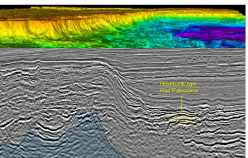
9. One of many leads (Rosebank type) interpreted as Paleocene sands between thin lava flows. These are found in front of the volcano-clastic delta sitting over the Møre Marginal Plateau. Soft anomalies and potential flat spots defines this multi layered lead. Shaded in blue is the rotated fault geometries observed sub-basalt. Inset in the top shows top basalt escarpment along the Møre Marginal Plateau.
