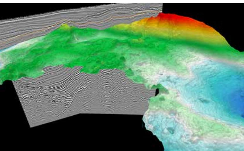
10. The Rân Ridge is interpreted as an uplifted Triassic-Jurassic depocenter sealed by the Base Cretaceous Unconformity. Between the highs we interpret entry points for Palaeocene gravity fan complexes with a proximal position around the Rân ridge. Tilted fault blocks are controlled by a decollement layer. The depocenter is reachable by exploration wells. 3D view shows Top Cretaceous gridded horizon.
