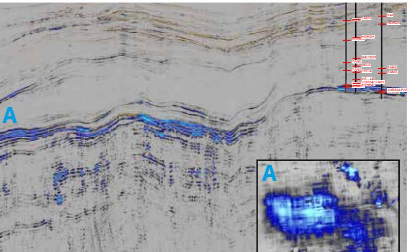
4. Arbitrary line within the TGS/Spectrum J-Cube tying the Ormen Lange field in the east (right) and out in the AM18 area in the west highlighting class 3 AVO trends (Far-Near\*Far, blue). The amplitudes within lead A show excellent correlation with the gas-filled Eggå sands in the Ormen Lange. Inset: Lead A indicates an anomaly in excess of  $300 \text{ km}^2$ .
