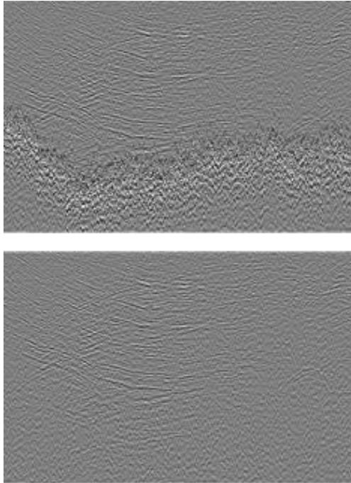
**Figure 3:** Un-migrated stack data before (top) and after deblending (bottom).
