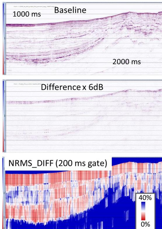
**Figure 2:** Baseline image of a single 2D line (top), Difference between co-processed monitor and baseline scaled by 6dB (middle), NRMS of the difference (bottom) using a 200 ms gate.
