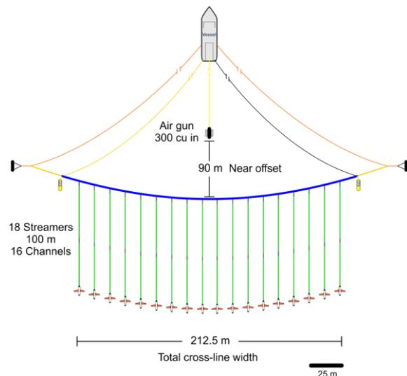
**Figure 1:** The P-Cable system layout consists of vessel towing an air-gun source and 18x 100 m hydrophone cables.
